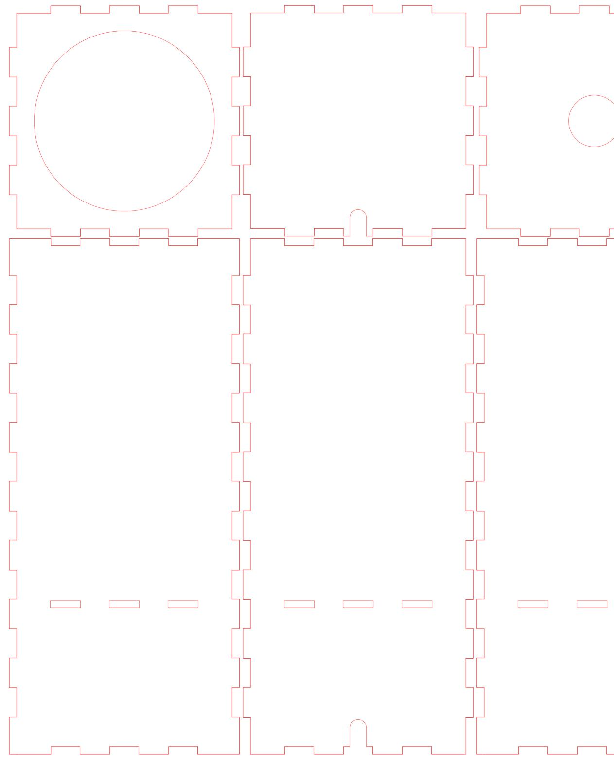
State Library of QueenslandLaser Lamp Squaremm height exc. base and lid4mm material thickness0.1mm kerf on holes80mm from base to middle holes
