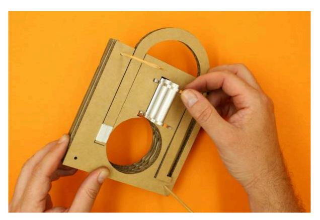
And slide the 3rd of our plastic Chamber Supports (the one with the smaller holes into the gap between the lower chamber support and the floor of the Chamber Assembly hole in the Hull Plates.
