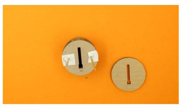
This front cover is 6mm, a bit thicker and cut out of the double-ply corrugated cardboard that the hull parts are cut from.
