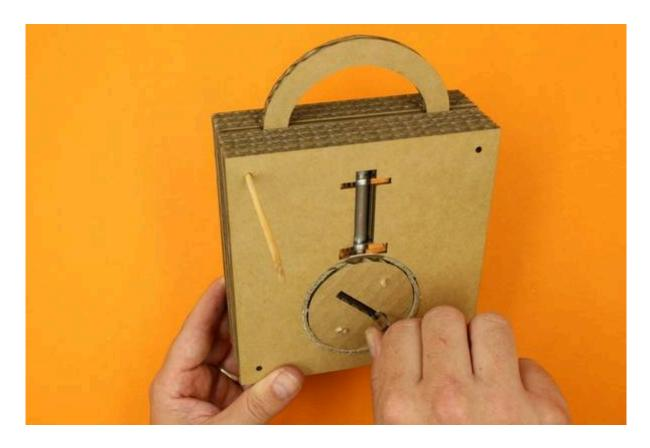
Once its in the 12 O'clock position and the pins are engaged, you should not be able to rotate the plug.
