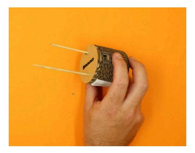
When you have that in place, trim the skewers to the required length with the side cutters. *Make sure you hold on to the bit you're cutting so it doesn't fly off and take out an eye!*
