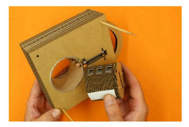
Orient the Plug so that the Key Pins and Plug Support are 90Deg from Chambers (9 O'clock Position). The Chambers should actually be lined up with your tape.
