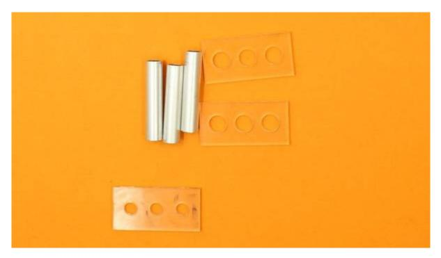
Start by fitting the middle metal tube into the centre hole on one of the plastic supports.
