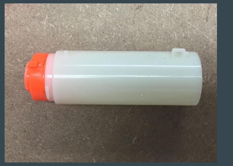
Attach air restrictor to plunger tube
