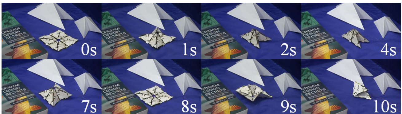
FIGURE 10. SEQUENTIAL STOP-MOTION PICTURES OF SELF-FOLDING, UNFOLDING AND REVERSE FOLDING VIDEO
