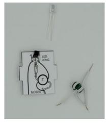
Insert the transistor legs through the holes.
