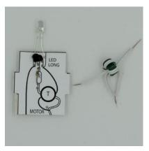
Bend over the last 5mm of the LED legs, and insert the LED beside the transistor. Twist onto the **side transistor legs** at the back.
