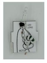
Insert the toroid wires, and twist the **joined wires** together with the **resistor** at the back, and
