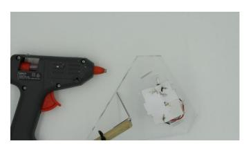
Bend the LED to fit into the hole provided in the chassis, and glue in place.
