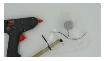
Slide the axle through the slot (motor hole to the left), and zip-tie in place.
