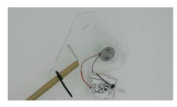
Attach the motor wires to the Joule Thief by pushing them through the template, and twisting
