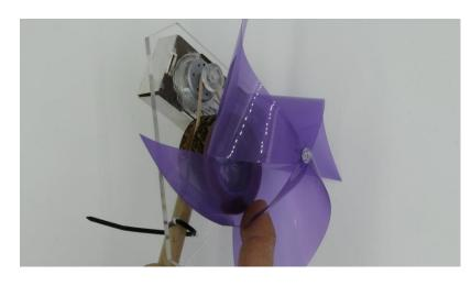
Blow on the spinner, and slide the handle up and down until it turns easily, but still moves the motor shaft.
