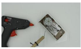
Insert the tabs into the slots on the chassis, and glue into place.
