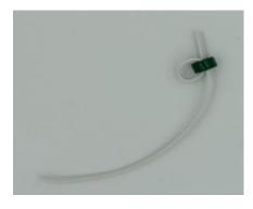
Take the 150mm piece of twinned wire, and loop it through the toroid.
