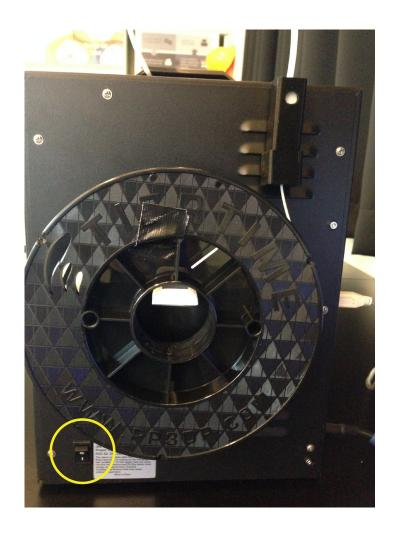
Turn the machine ON. The switch is located on the back of the machine, bottom right hand corner.
