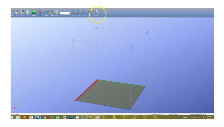
Should any errors occur while you are printing you can always stop the print by hitting the 'Stop' button in the Up Software
