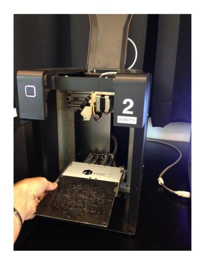
Insert a clean perforated bed into the 3D printer. Remember to use two hands and be careful not to put too much force on the printing bed platform.
