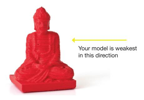
If you are planning to make a structural part on the printer you may want to consider rotating the model to give your model optimal strength
