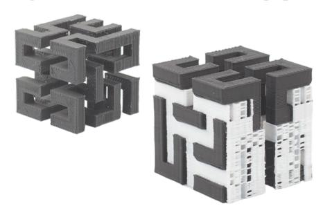
Any overhangs in your 3D model which exceed 45 degrees will require a temporary support structure to hold up the molten plastic during printing. The supports generally print as a disposable structure which will easily break away from your model. Some 3D printers will automatically insert these supports for you, others will require you to manually insert these in your 3D drawing. Support can be disabled by changing "Area 7" to "Only Base"
