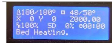
The printer first waits for the bed temperature to reach the target temperature
