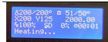
The printer will then wait for the nozzle target temperature to be reached
