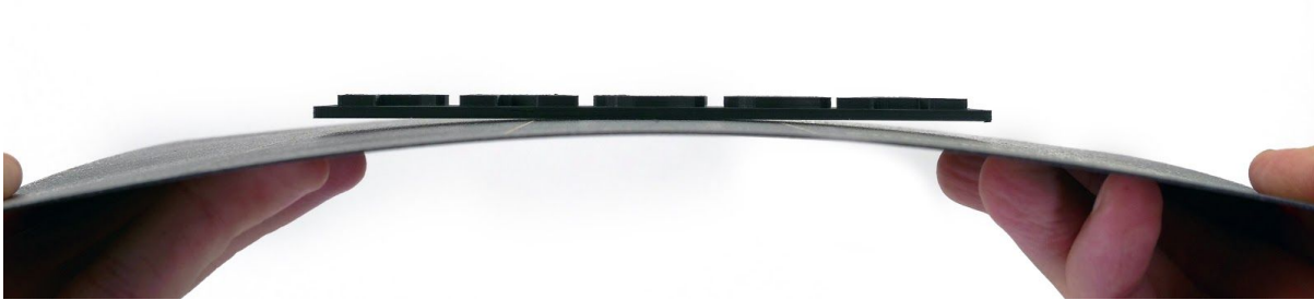
Pict. 13 - Removing the model from the PEI print surface by bending the steel sheet.
