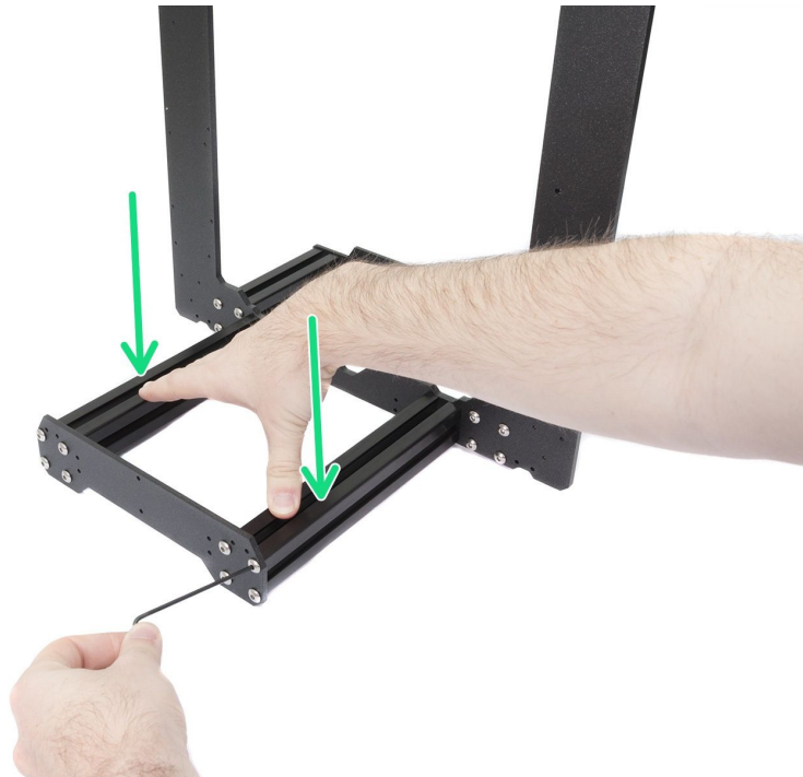
Pict. 46 - Proper way to tighten the frame, plates and aluminium extrusion together.
