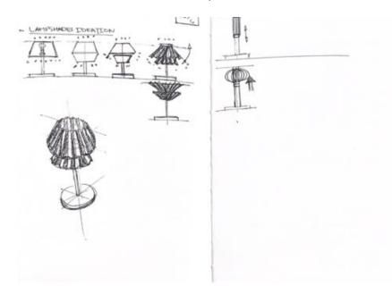
The lampshade uses a pattern similar to how a simple origami fan is constructed with angled folds to create a flare in the lampshade profile.
