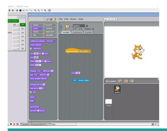
Drag the sensor value block into the say block, and the sprite will begin to 'say' the sensor reading on the screen (many times a second).
