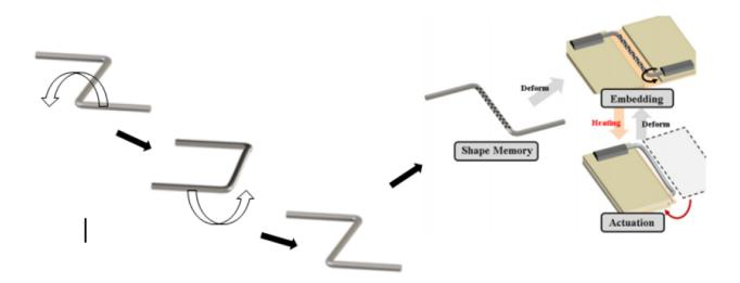
Heating causes the wire to untwist, and any segments attached to the legs will be rotated (see: <a href="https://youtu.be/wzM0hxsg2VE">https://youtu.be/wzM0hxsg2VE</a>). Attaching two twisted elements that turn in opposite directions will allow for more rapid recovery when each is heated alternately.
