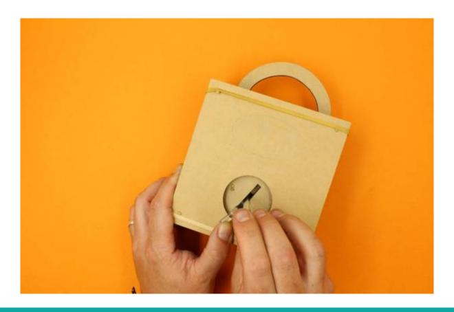
If you are doing this correctly the torque on the plug should provide a small ledge for the set pin to rest on at the "Shear Line".
