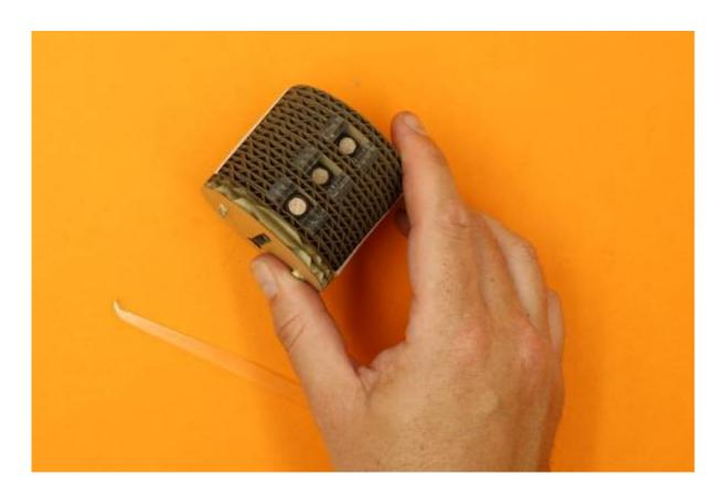
and check their function (i.e. that they move up and down freely) by manipulating them using you pick via the key hole
