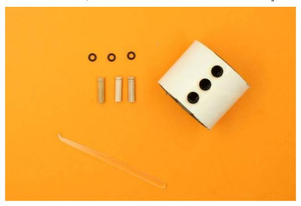
The key pins are the three shorter dowels (24mm long) with a groove cut into them. Seat the Orings on to the three key pins
