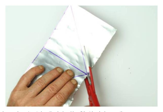
Use heavy scissors to cut along the sloping sides of the triangle drawn on the can.
