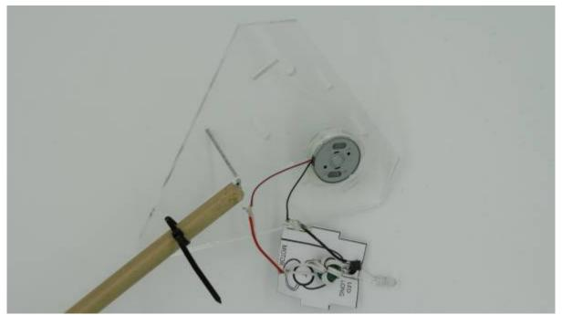
Now attach the motor wires as indicated: black wire to the transistor + LED, and red wire to the joined toroid wires.
