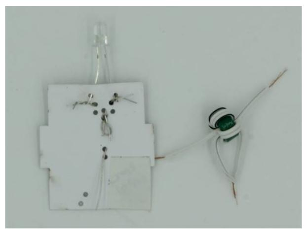
Attach the LED, taking care to put the longer leg on the right side. Twist together with the transistor on the back of the template.
