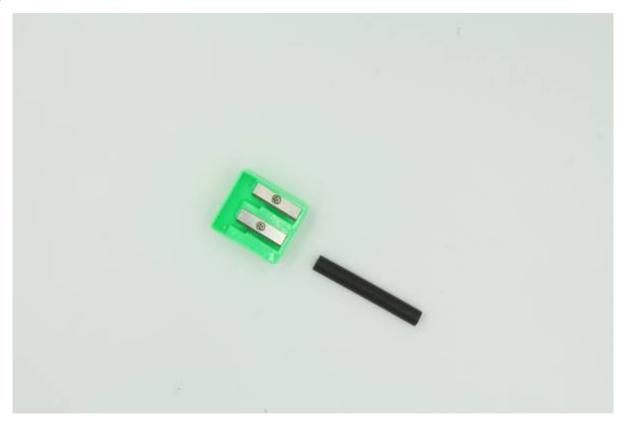
Cut a piece of tubing 10mm long. This will act as a spacer to hold the spinner hubs in alignment with the motor. Sharpen one end in a pencil sharpener before cutting it off. Trim the ends flat with a craft knife if necessary. Sharpening the end reduces friction with the acrylic hub, so make sure this end is towards the hubs.
