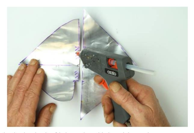
Use hot glue along the edge of the bottom piece to join the two halves together.
