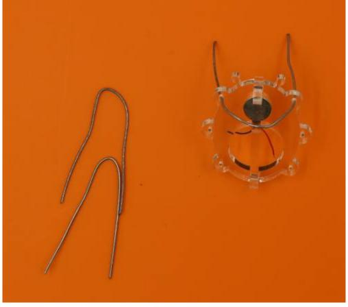
Bend the three pieces of wire in the middle. Insert through the holes in the body FROM THE BOTTOM as shown.
