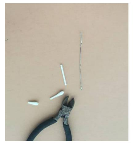
Cut the ends off the cotton bud, and check it is hollow, and that the straightened wire will fit easily down the centre. Some extra straightening might be needed, and the smoother the fit the better.
