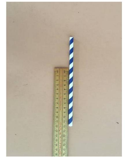
Cut the paper straw to a length of about 13cm. Scissors tend to crush the straw, and a boxcutter gently used like a saw will work better, especially if you work your way around the straw cutting one side at a time.
