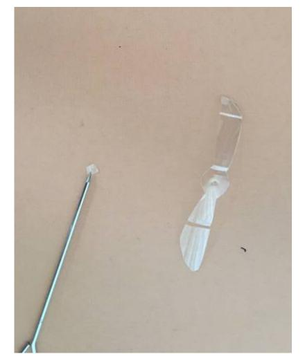
Cut a small circle of plastic from the PET bottle - this needs to be less than the diameter of the propeller hub, 6 or 7mm diameter if you can manage it. It does not matter if it is not very circular.
