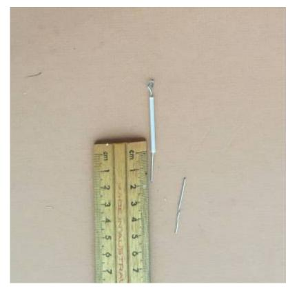
Slide the wire axle through the shaft bearing, and check it can rotate smoothly.
