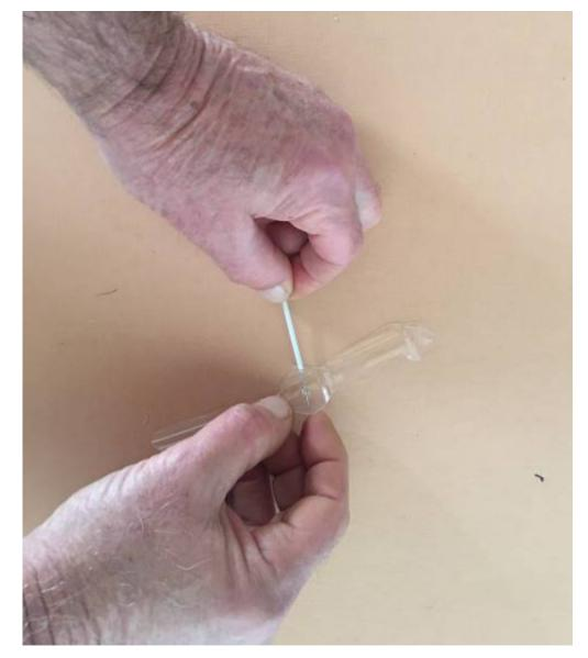
Slide the washer onto the propeller axle, and then the propeller. If your skewering has raised one side of these pieces, then place the two smooth sides together to minimise friction.
