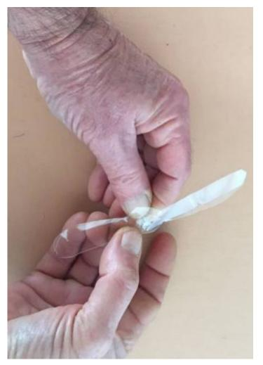
Push the propeller down the shaft, and use the pliers to bend the protruding shaft into a U-shape, with the open end of the U facing the propeller.
