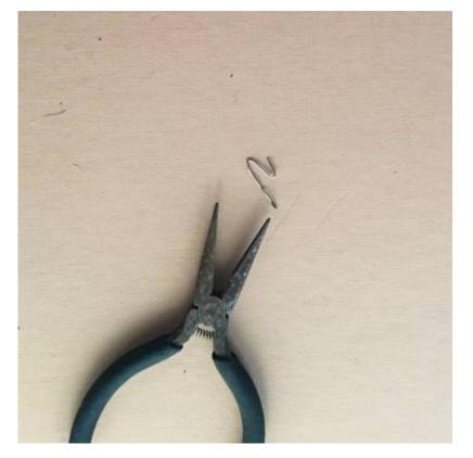
You will need a hook at the end of the straw to hold the rubber band, but it is best fixed in place later (alignment is important). Bend the tail hook into an Z-shape, as shown. The longer tail will slide inside the straw, to help keep the hook in place.
