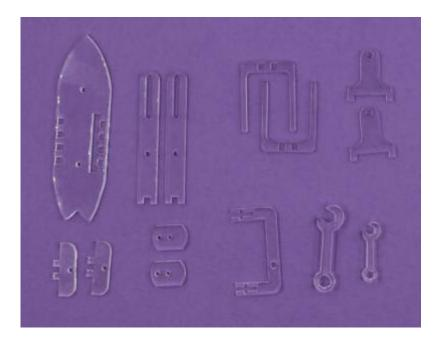
Peel plastic off laser cut parts
