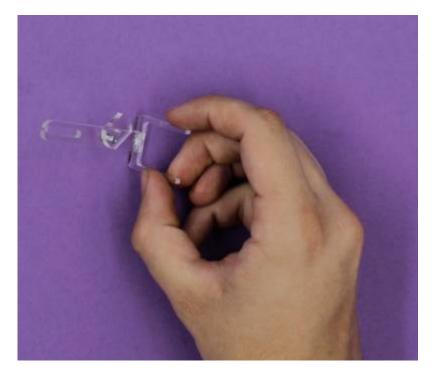
Attach the small gear (m) to the motor (I) carefully as the shaft is keyed with a D shape on the opposite side to the winder
