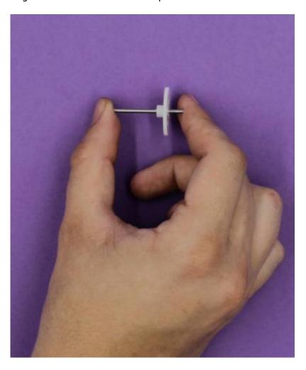
Place the D shaped pieces (e) on the shaft and apply a small amount of glue to the tabs
