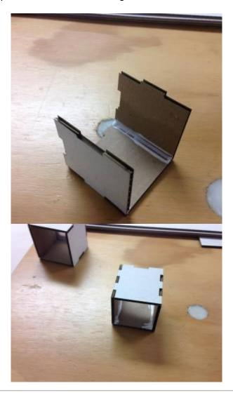
**5.**Slot the B panel into the grooves at the back of the inner box and fix with glue.
