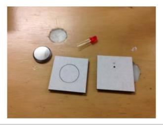
2. Slot the LED contacts into the E panel with the longer contact in the outer most hole and place the coin battery into the hole of the F panel (Negative side up).
