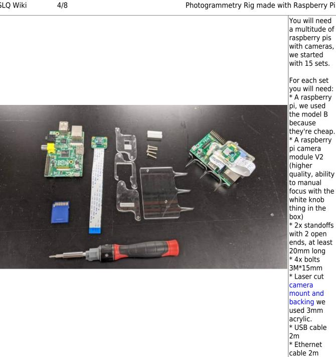
For each set you will need: \* A raspberry pi, we used the model B because they're cheap. \* A raspberry pi camera module V2 (higher quality, ability to manual focus with the white knob thing in the box) \* 2x standoffs with 2 open ends, at least 20mm long \* 4x bolts 3M\*15mm \* Laser cut camera mount and backing we used 3mm acrylic. \* USB cable 2m \* Ethernet cable 2m
