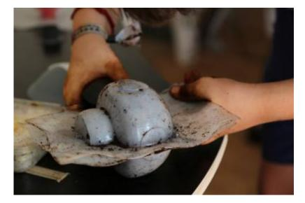
Moulds vacuum formed from sheet plastic can now be stapled together around the edges.
