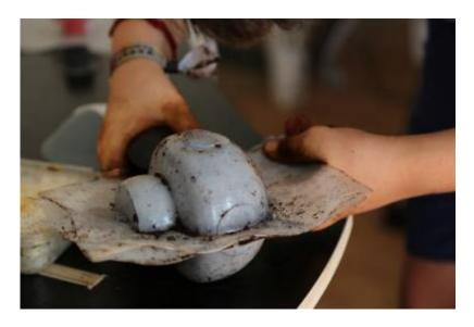
Moulds vacuum formed from sheet plastic can now be stapled together around the edges.
