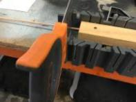
Press inside face of the saw blade against the inside surface of the 90 deg mitre box gap. Use a square to measure the desired length (in this case 25 and 30mm) Secure a block of wood as a stop. As you cut check your tolerances regularly.
