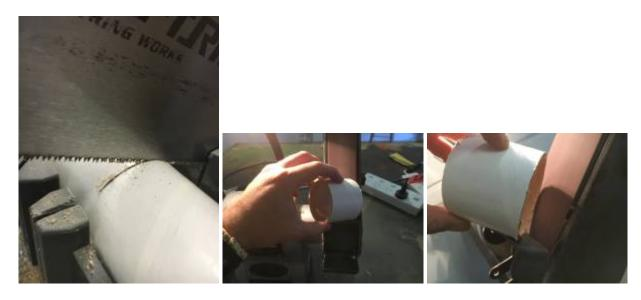
Clean up daggy edges on sanding belt on the bench grinder. Use the workrest on the belt sand to level up the cuts to 90 deg
