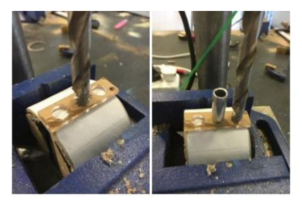
after drilling each use metal sleaves to ensure the alignment of the hole template is correct
