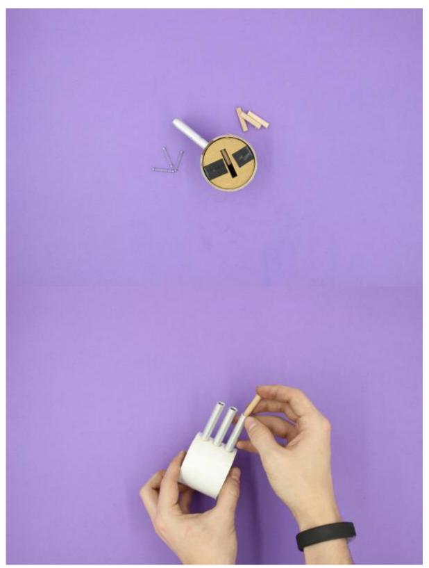
Grab the chamber support and put it over the chambers, the open end should be facing to the front of the plug/lock. It is important that you don't press the chambers into the actual plug, as it won't turn. Once the support is in place (you may need to hold it due to the tension from the springs), gently squeeze your plug housing and chambers into the hull, there should be some resistance so try wiggling in.
