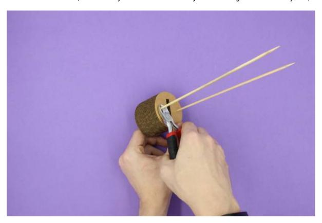
Grab two of your magnets and insert them into the small hole on one of the sides of your plug. Face the magnet front/back outwards. Make sure it is lower or flat with the surface otherwise it may cause unwanted friction when turning the plug. It doesn't matter what direction the polarity is going for the time being. We will match the other magnets with it later.
