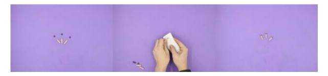
Finally, insert the key pins into the holes in the plug keeping the end with the o-ring pointed up, our acrylic rings should keep it from falling too far down. It should be easy to push the pins up and fall back down when released. You can use your lock pick or tension wrench to test it out. If you are having problems you might need to adjust your rings.
