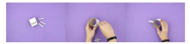
Put the plug into the housing and twist it 90 degrees. We do this so we don't accidentally push our chambers into the holes in the plug.
