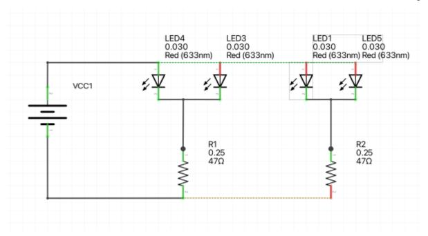
Positive accross the top and negative from the bottom via each of the resistors
