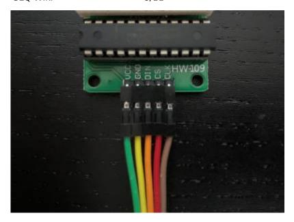
In the example above, VCC on the LED Matrix the cable is Green which would be connected to the VIN pin on the Arduino.
