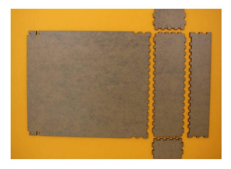
Lay out the pre-cut pieces for the moss wall, and remove the protective paper coating from the INSIDE only.
