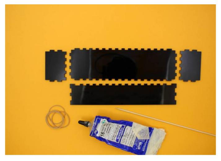
After removing the internal protective paper from the bottom tank parts, assemble acrylic glue, skewer (for spreading glue) and rubber bands (to clamp the assembled job).
