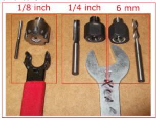
• While pressing down yellow 'Spindle Lock' button, loosen collet to remove previous tooling.
