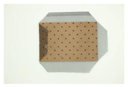
Continue folding and gluing down the mesh until the pegboard is covered, and make sure that it fits snugly inside the frame before continuing.
