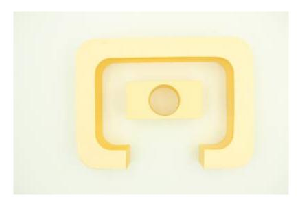
One piece of the 50mm foam has a circular hole cut to take the vacuum cleaner hose. The hole diameter should be such to give a snug fit around the ribbed hose - not one of the nozzles - because while nozzles vary between brands, the hose is usually standard at 39mm external diameter. Making the hole a bit smaller is OK, since the foam is soft and the hose can be twisted in to make a good fit. If a loose fit is found, wrapping the end of the hose with tape can make the connection airtight.
