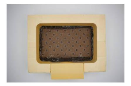
Turn the assembly over, and check again that the frame will fit snugly over the pegboard now that it is fixed in place.
