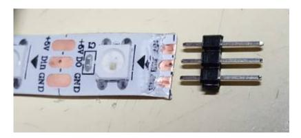
• Tin contacts to ensure they are clean, tin short end of connector. Solder connector in place. Using a socket of some kind helps keep them aligned.
