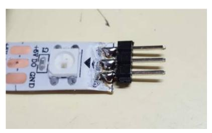
• Cover the soldered end from the lettering up and including the plastic base of the header with neutral cure silicon.
