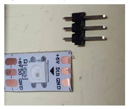
• Some waterproof strips have a cover, cut and peel back the last few mm to expose bare copper.
