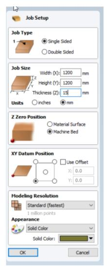
Make sure your material dimensions match your Job dimensions. For the inductions we use use a 2400x1200x17mm sheet. Measure all dimensions on the sheet!
