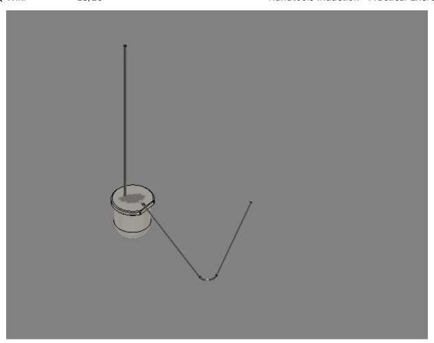
orient the LED so the short bent leg is *inboard*- towards the cell (battery) and the positive (+) long leg is outboard.
