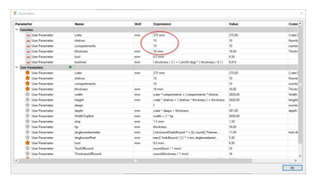
Check out the toolmax parameter value. It suggests I can get away with a tool up to 9.5mm (round it to the nearest .5 mm)
