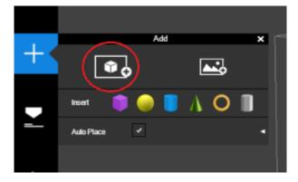
By pressing the + Button in the main menu you can add models, primitave 3D shapes or an image (which you can create a 3D model of). The model should show up in the 3D view area.
