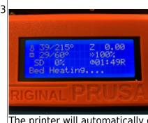
The printer will automatically commence heating the nozzle and the bed to the correct temperatures for the chosen filament; printing will start when the target temperatures are reached. This can take several minutes.
