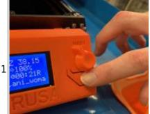
For a catastrophic failure press the **Reset (X) button**. This will abort the job and force a full reset of the printer.
