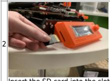
Insert the SD card into the slot on the side of the LCD screen assembly
