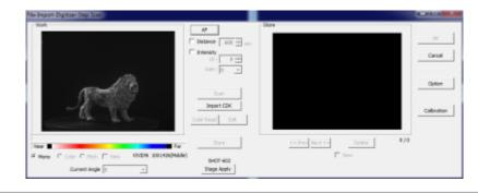
Hit [AF] to focus the camera/laser. It will make a little rustling noise. hit [scan] to test the laser. If you get an autofocus error, it's probably because the line of sight from the laser (at the bottom) to the object is obscured by something. click [Option] and in the window that appears, click [Apply]
