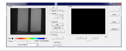
If it comes up with an error, or just a coloured scan, move the position of the turn table (with calibration chart on it) and try again.
