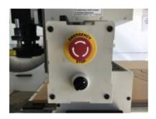
This can be activated to bring the machine to an immediate stop in an emergency.
