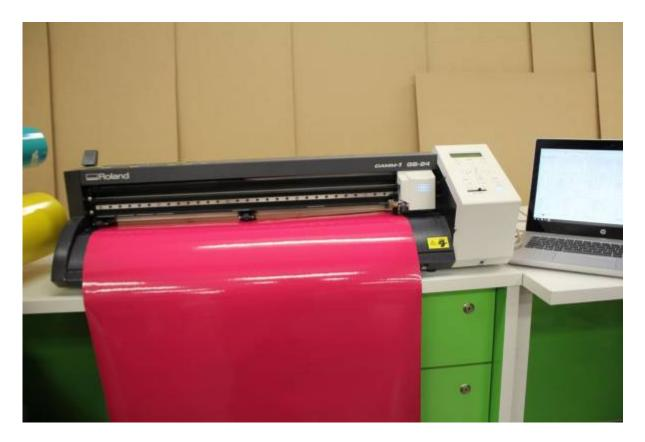
The GS -24 vinyl cutter is a popular piece of equipment in the Fabrication Lab that is relatively easy to use and can make a big impact. Over the year members of the public and the Fabrication Lab team have used it to make also sorts of stuff that can cut a range of materials
