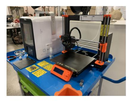
**Printer type:** Fusion Deposition Modeling
