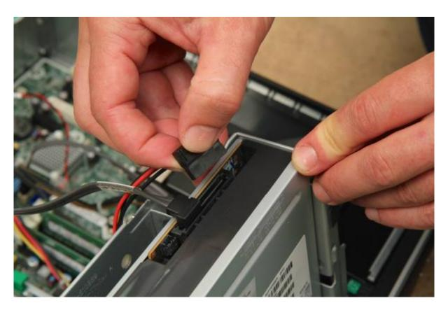
Ensure cables run through the cable clip.
