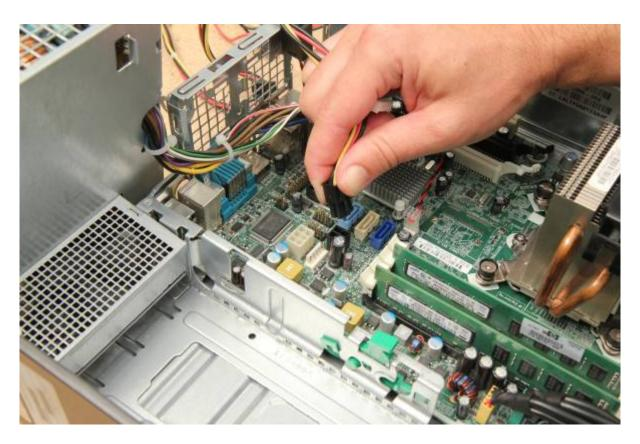
Clear the cables, then tilt the PSU and lift straight out.
