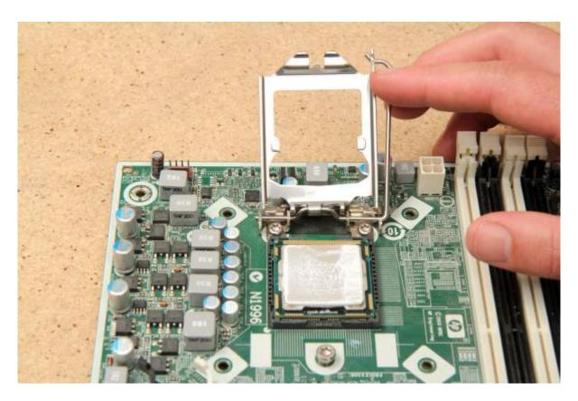
Carefully remove the CPU with two fingers, from the edges with small notches in the socket.
