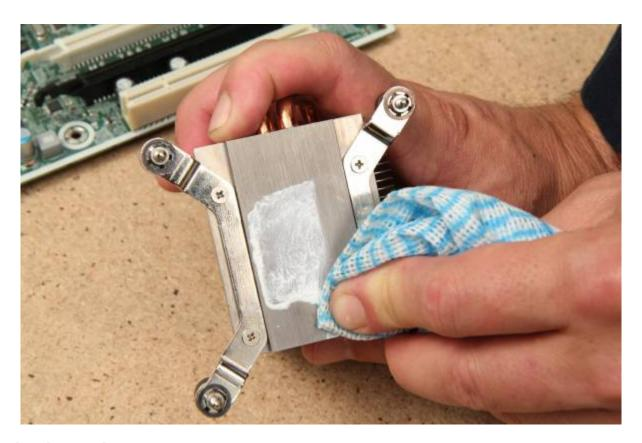
**Apply Thermal Paste/Reseat CPU**
