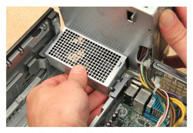
Re-connect the PSU cables to the motherboard (they only fit one way).
