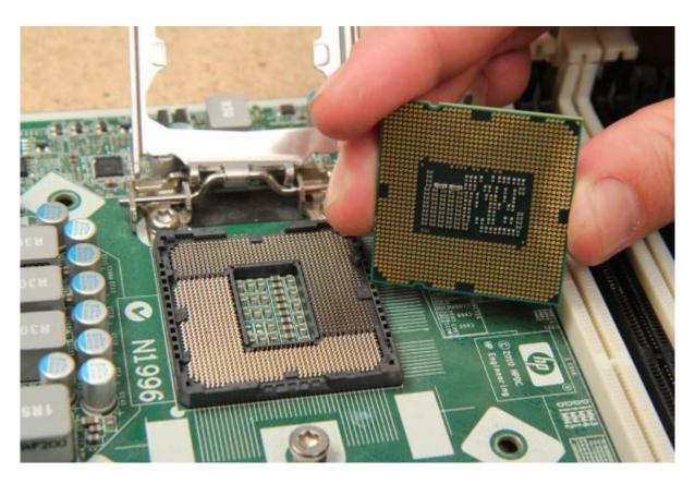
Hundreds of pins each connect to a gold circle on the base of the CPU.
