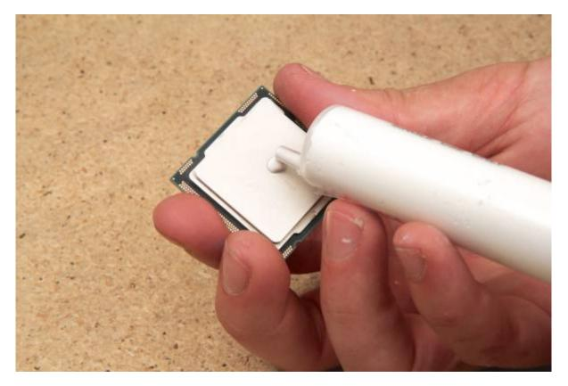
Flip and smooth the paste onto the heatsink until the CPU is mostly covered (not essential)
