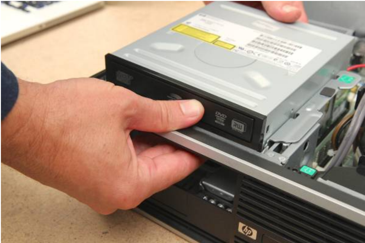
The drive label contains information to help replace/upgrade the drive.
