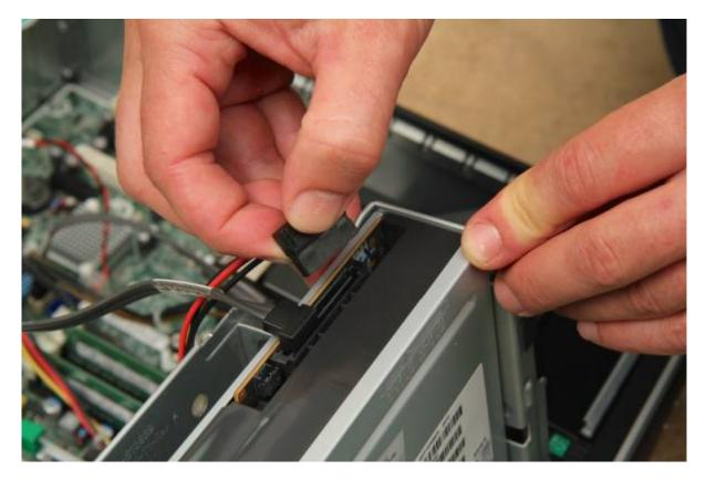
Ensure cables run through the cable clip.
