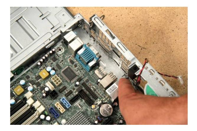
Lift and twist to clear from the case. Lay in a clear space.
