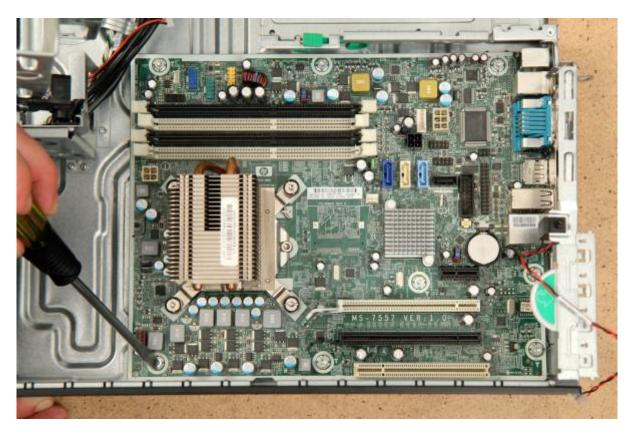
When removing the heatsink do not touch the sticky paste on the heatsink/CPU. This thermal paste improves heat transfer between these components.
