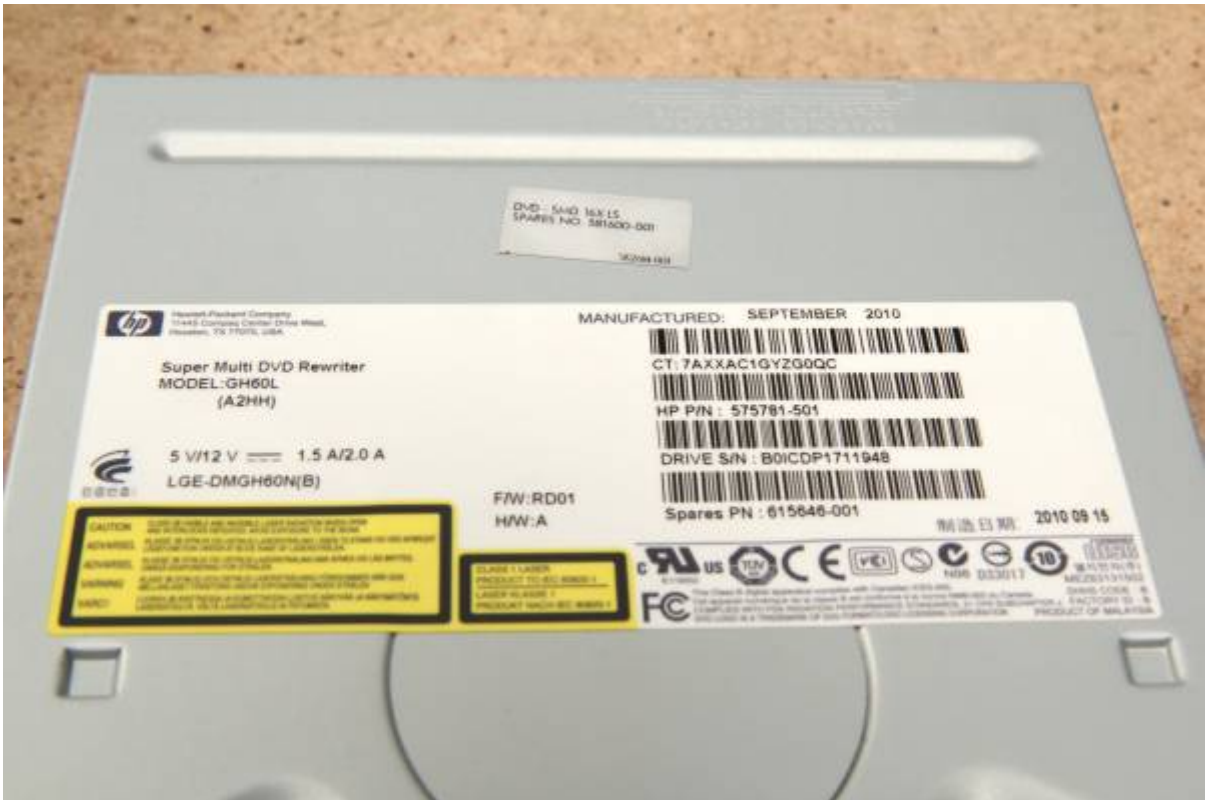
The drive label contains information to help replace/upgrade the drive.
