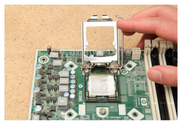
Carefully remove the CPU with two fingers, from the edges with small notches in the socket.
