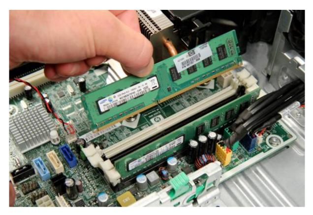
Don't touch the gold parts on RAM, as skin cells/sweat can cause corrosion
