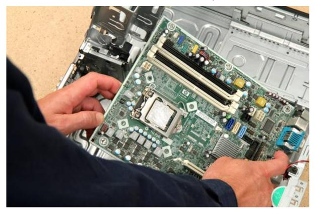
Replace and tighten the six screws (don't use heatsink screw holes).
