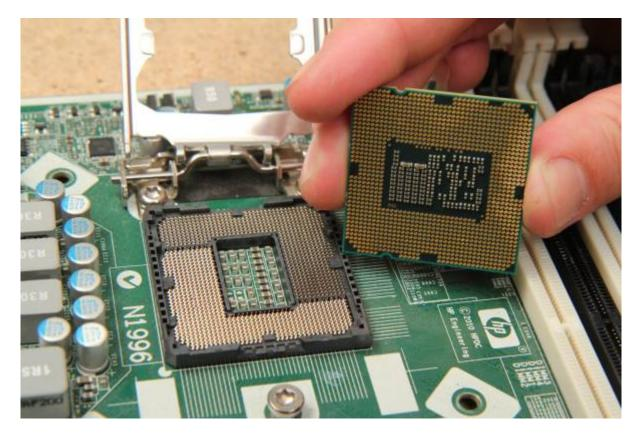
Hundreds of pins each connect to a gold circle on the base of the CPU.
