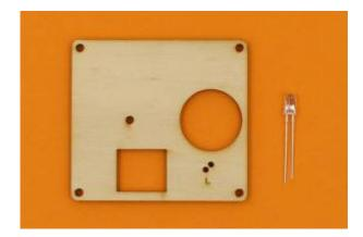
The LED legs go through the two smallest holes on the middle board, and the long leg hole is marked with an "L".
