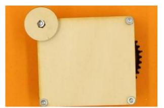
You may need to press down firmly on the bottom plate to attach nuts to the corner screws (pressure also helps keep the motor support in place). Use the wooden spanner to tighten the nuts.
