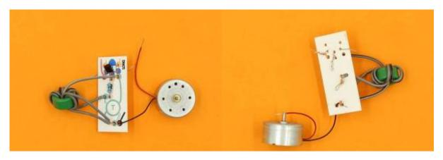
Now take the red wire on the motor, and push it through the hole at the end of the **red** line on the circuit.
