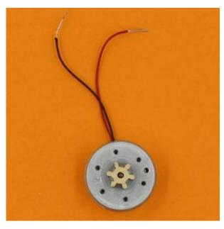
Take the black motor wire through the hole at the end of the **black** line on the circuit. It comes through next to the joined toroid wires, and you can twist all these together. (The cog is missing from the following images, but should already be on your motor)
