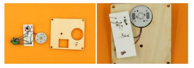
As you can see, the motor fits into the round hole, and the toroid will fit into the rectangular hole when everything is in place.
