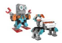
Jimu is a great introduction to robotics and coding, with easy to follow instructions, you can use a tablet to move the robot around, record and playback poses and detect objects using its infrared sensors.
