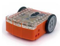
An Australian based robot which is LEGO compatible, the Edison can be converted into a myriad types of machines with the EdCreate extension pages, LEGO blocks, or whatever you might have lying around! Edison can be coded via its own block-based coding language - EdBlocks, or via barcodes, and can be driven with any infra-red remote control unit.
