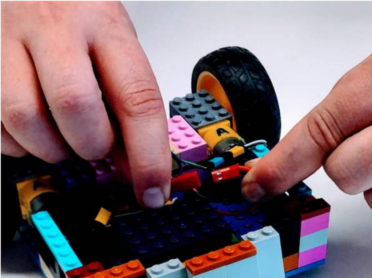
**4.** Now it's time to test that the instructions from the Arduino is being sent to the right place. You'll know that the pins have been plugged in correctly if the Robot Racer drives in the correct directions when controlled using the Playstation style controller.
