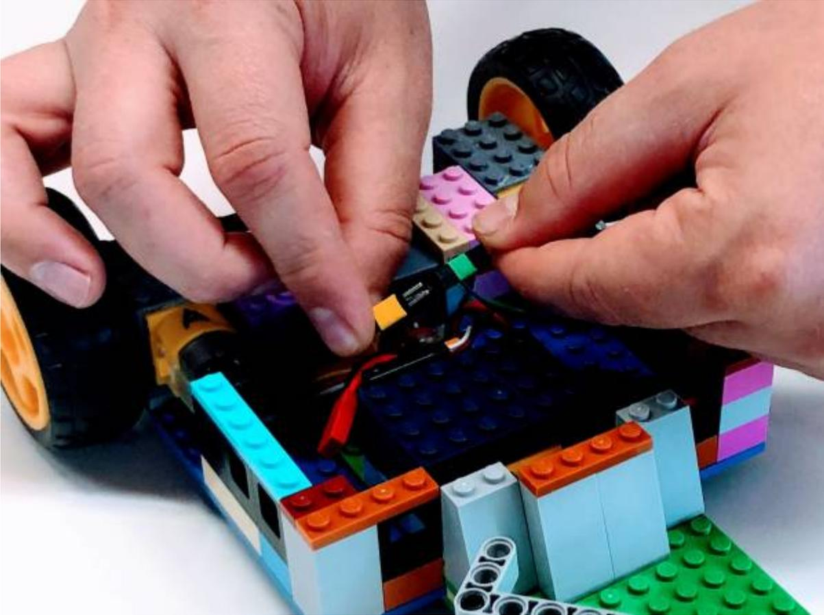
**2.** Plug the other motor cable with the YELLOW pins into the wire with the BLUE plug. Now both your motors are connected.
