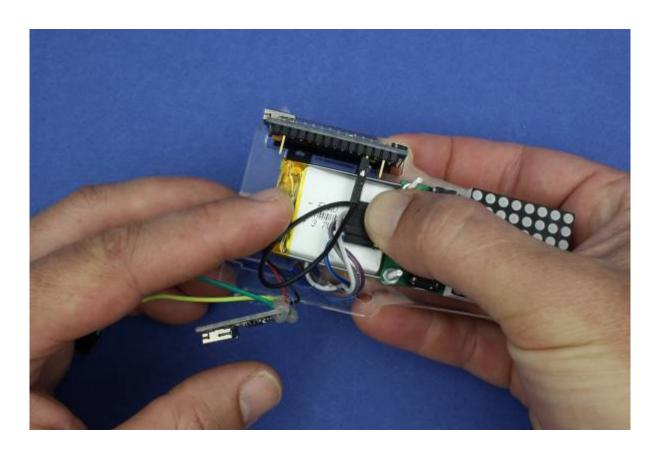
Slide the USB charge board into the slot
