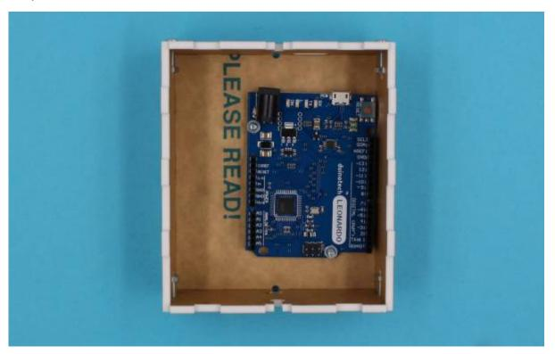
Finally put the top piece of the case on. If you're having issues try loosening a couple of the bolts of the case for some more wiggle-room.
