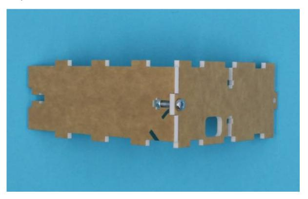
Put the two assembled sides with your base and see that everything aligns. Take note that the USB port should be perfectly aligned with the hole in the front piece of the case.
