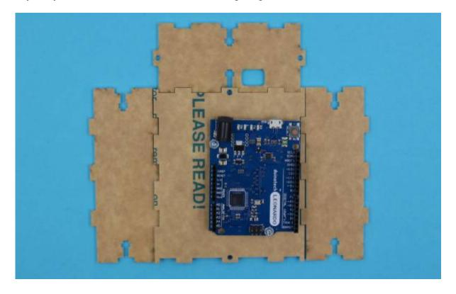
Take the front piece of the case and one of the sides. Note where the nut and bolts go.
