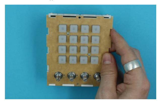
Add two nuts and bolts to the front, fixing the base and top to the sides.
