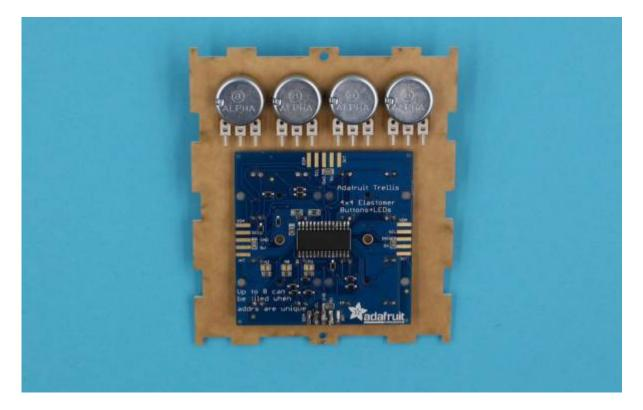
Use the two smaller nuts & bolts (1.5mm) to attach the Trellis board to the case.
