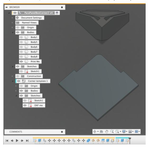
The a STL design for the corners and a *DXF* for a corner cutting template can be downloaded after entering your card thickness into the parameters
