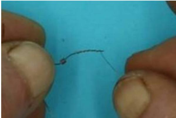
Slide the crimp along over the top of the wound copper, and crush it closed using pliers. Give the copper wire a gentle tug to make sure the crimp is holding it in place securely.
