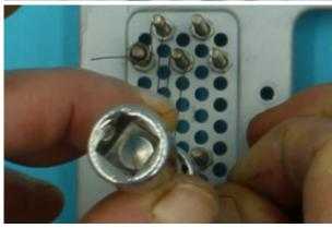
Now the memory wire is constrained in the shape required, proceed to the heating.
