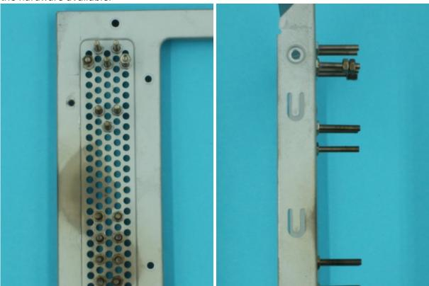
Each retainer post consists of a 3mm machine screw held in place with a nut.
