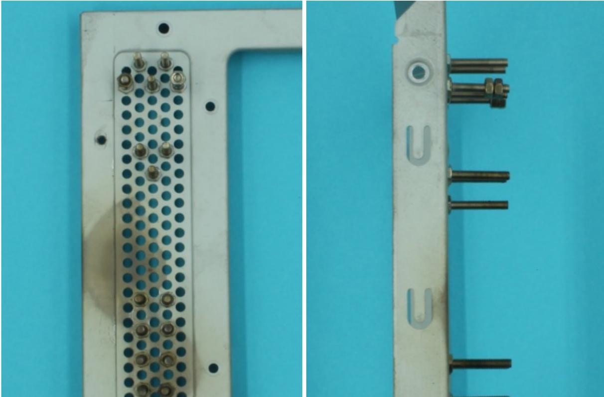
Each retainer post consists of a 3mm machine screw held in place with a nut. Attachment points for the wire are made by attaching two more nuts to the top of the screw. The wire is inserted between the two nuts, and held there while the top nut is tightened to jam it in place as shown below.
