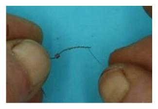
Slide the crimp along over the top of the wound copper, and crush it closed using pliers. Give the copper wire a gentle tug to make sure the crimp is holding it in place securely.
