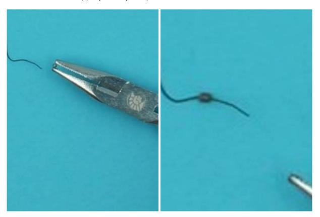
Slide the crimp along the wire so that the end is exposed, and wrap the end of a length of fine copper wire around it. You might need to bend the end of the copper wire over to lie along the memory wire to achieve the next step.
