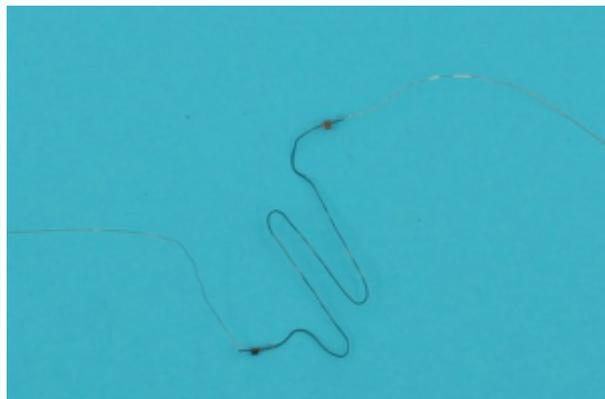
NOTE: At this stage it is important to retain the trained shape of the memory wire so that it can be inserted correctly into the design. This example will change from straight to the concertina shape shown, but the change only happens along one plane, and this has to match the required movement of the piece attached.
