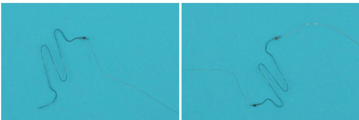
NOTE: At this stage it is important to retain the trained shape of the memory wire so that it can be inserted correctly into the design. This example will change from straight to the concertina shape shown, but the change only happens along one plane, and this has to match the required movement of the piece attached.
