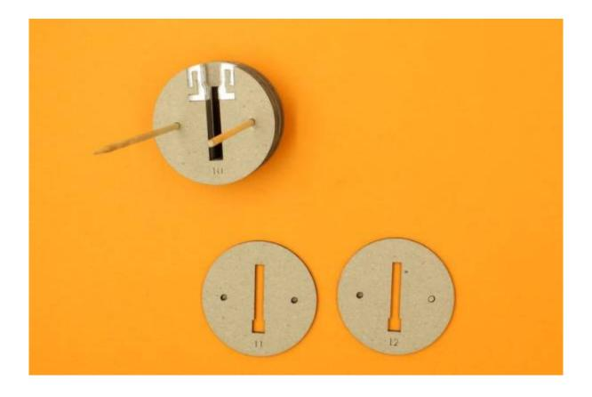
Now add the last three layers of plug plates and the two plastic plug supports for each layer
