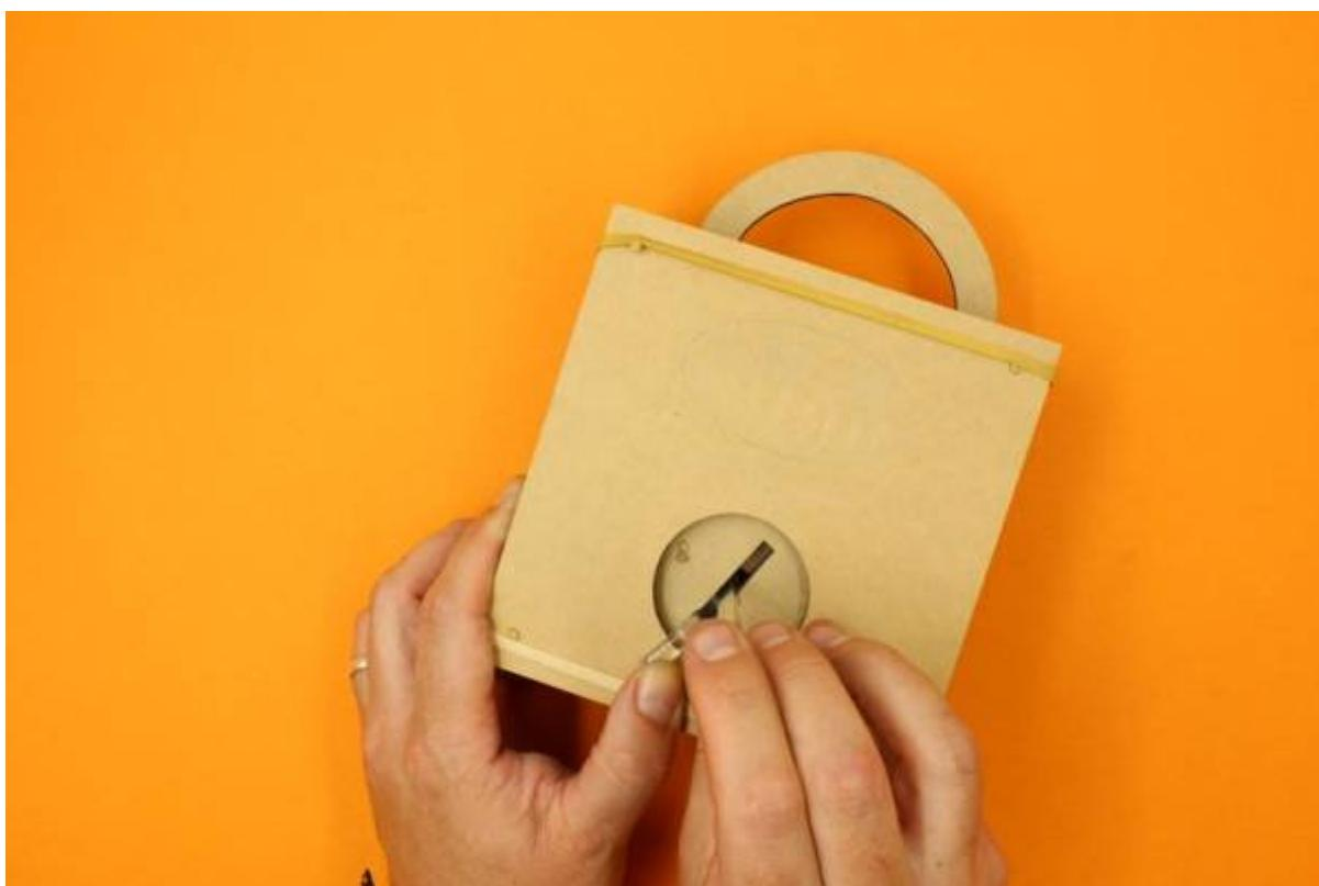
If you are doing this correctly the torque on the plug should provide a small ledge for the set pin to rest on at the "Shear Line".
