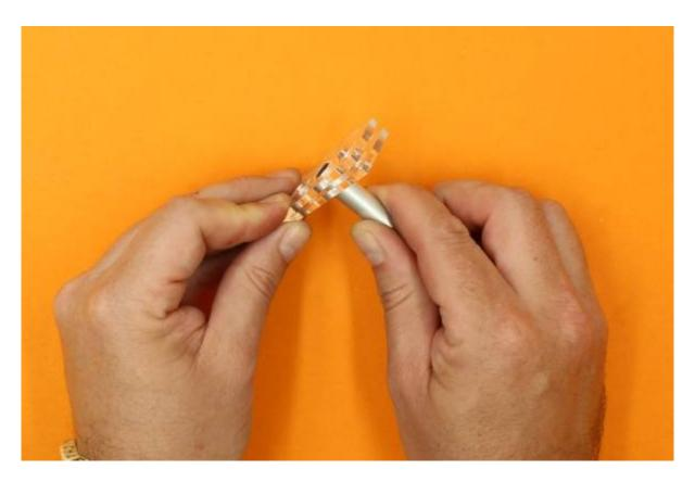
Align the outside holes of the plastic chambers supports and fit the other two metal chambers
