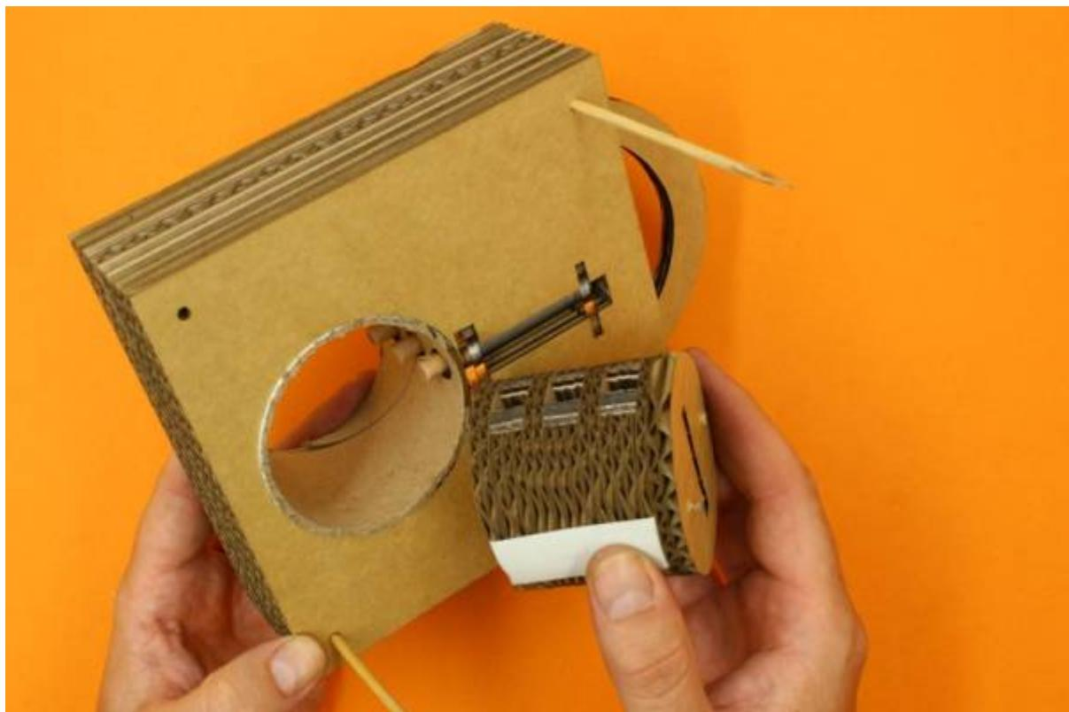
Orient the Plug so that the Key Pins and the Plug Support are at 90 degrees from the Chambers (i.e. 9 O'clock Position). The Chambers should actually be lined up with your tape
