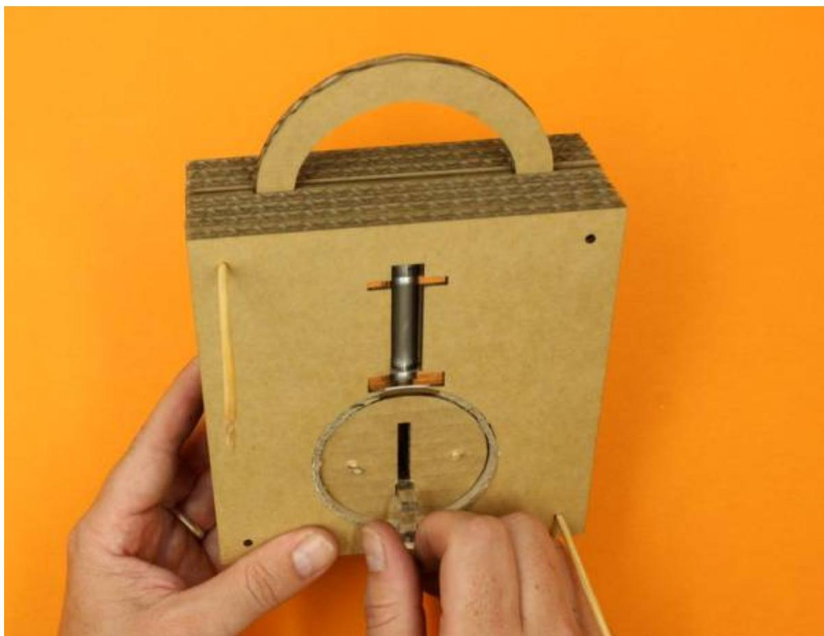
To pick the lock insert your tension wrench and use it to apply a slight rotational force (torque) to the plug
