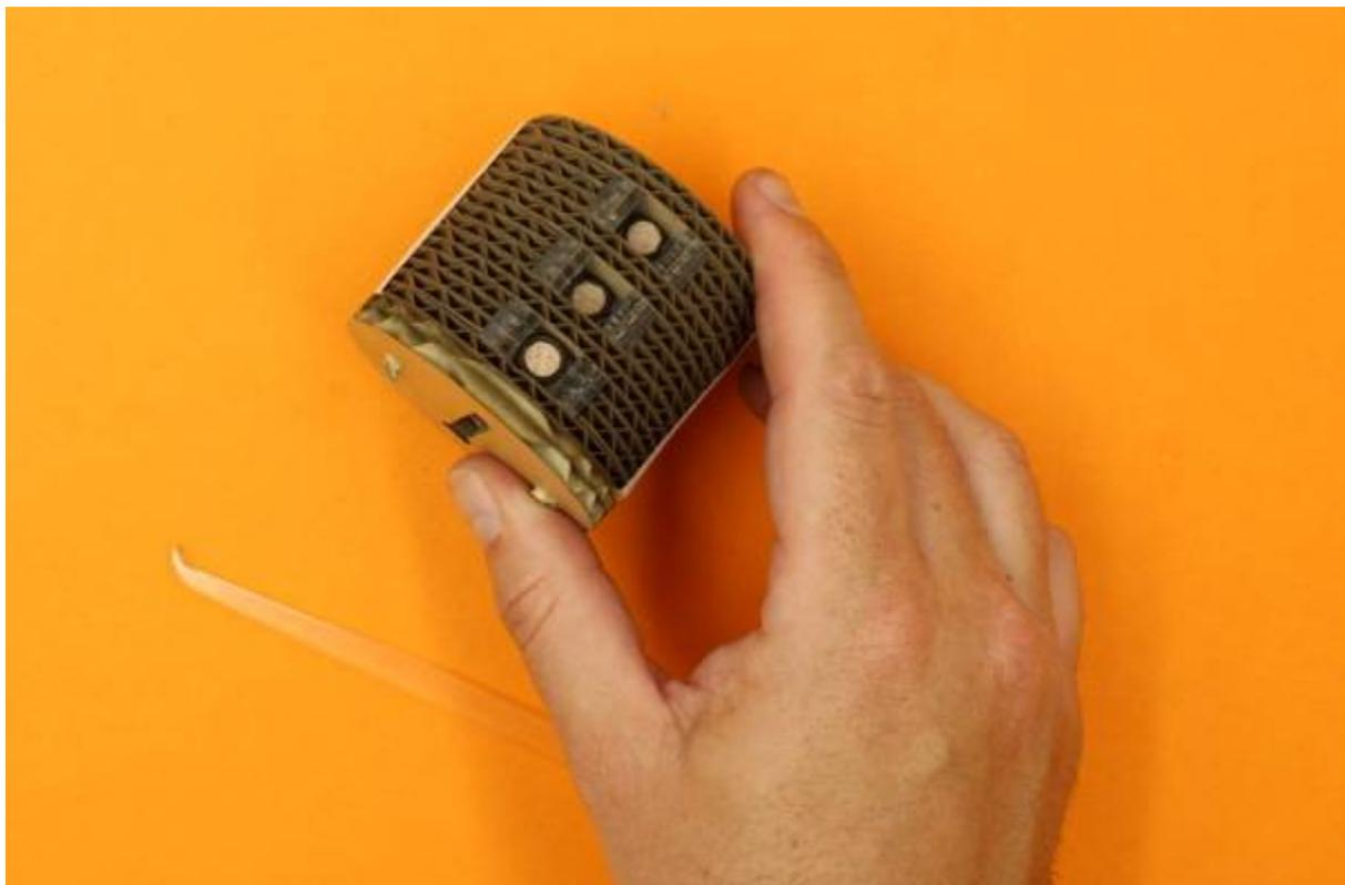
and check their function (i.e. that they move up and down freely) by manipulating them using your pick via the key hole
