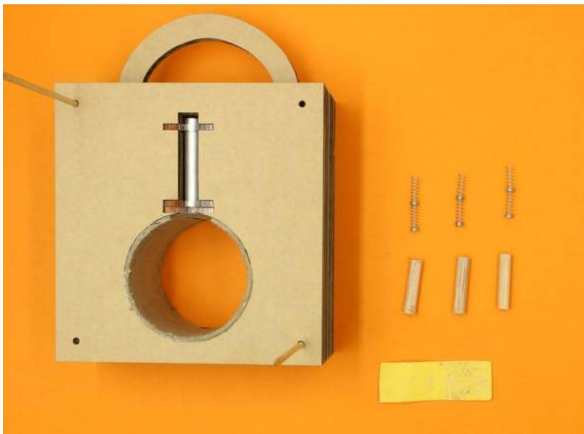
First deburr the **set pins** using the piece of sandpaper to ensure that they move freely in their chambers
