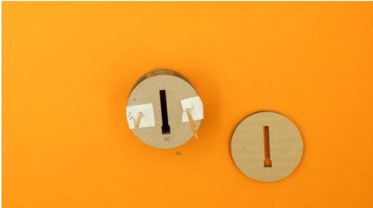
This front cover is 6mm, a bit thicker than the other layers, cut out of the double-ply corrugated cardboard that the hull parts are cut from
