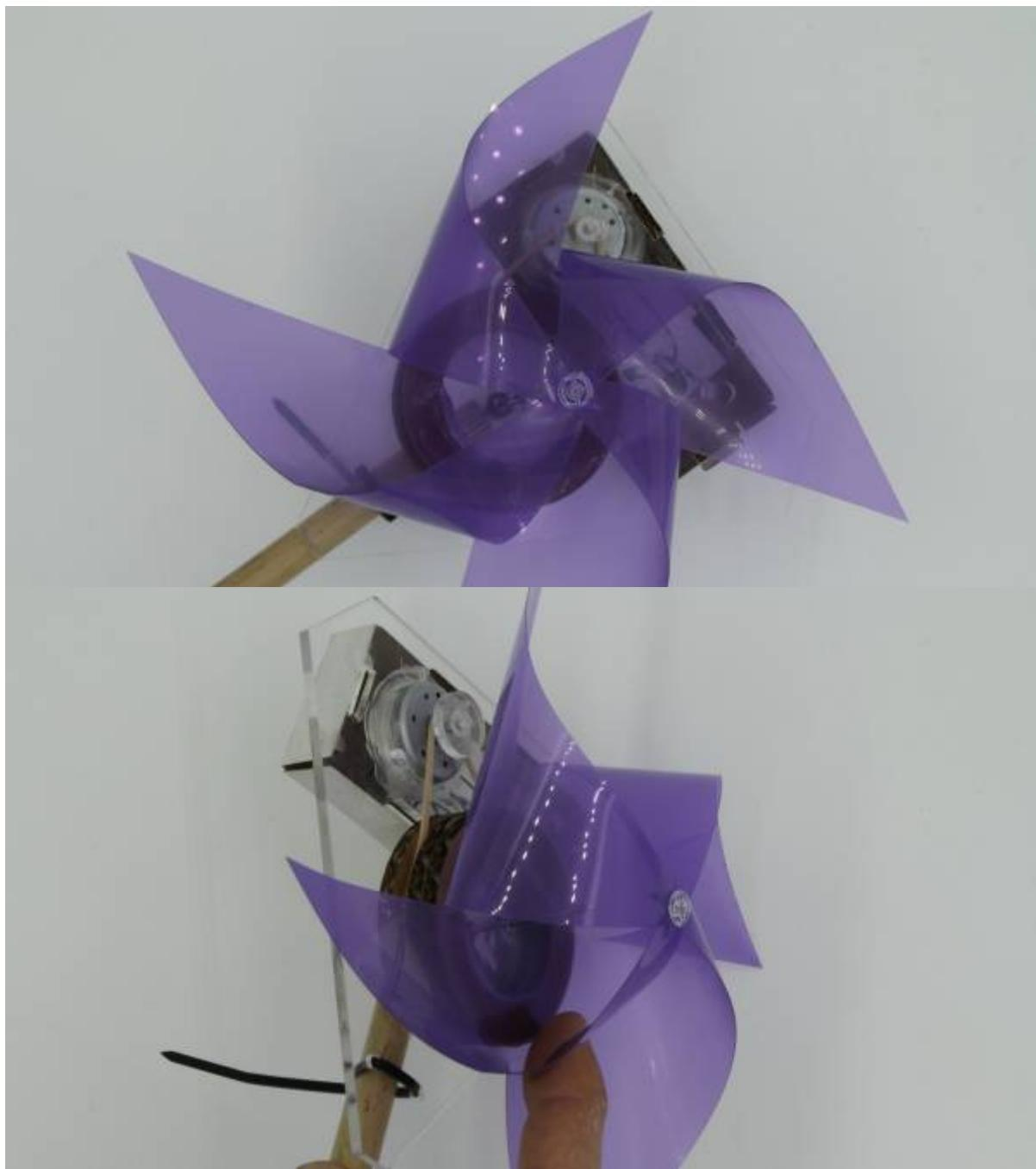
Take the rubber band, and loop it over the hubs so that it sits in the groove made by the acrylic hub. Now slide the 10mm spacer on to the axle, and then the spinner with the double hubs closest to the chassis.
