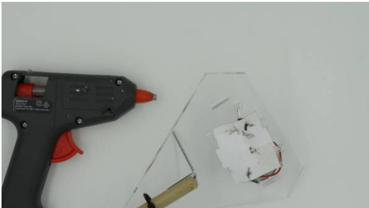
From the back of the chassis, insert the LED into the hole provided, and glue it in place.
