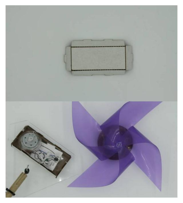
First, fold the enclosure along the scored line. Now fold and fit the tabs into the slots in the chassis, enclosing the circuit.
