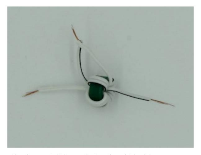
The toroid now has two pairs of wires emerging from either end of the winding.
