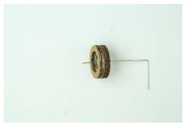
Thread the sandwich of hubs onto the wire assembly stand, with the double hub uppermost.
