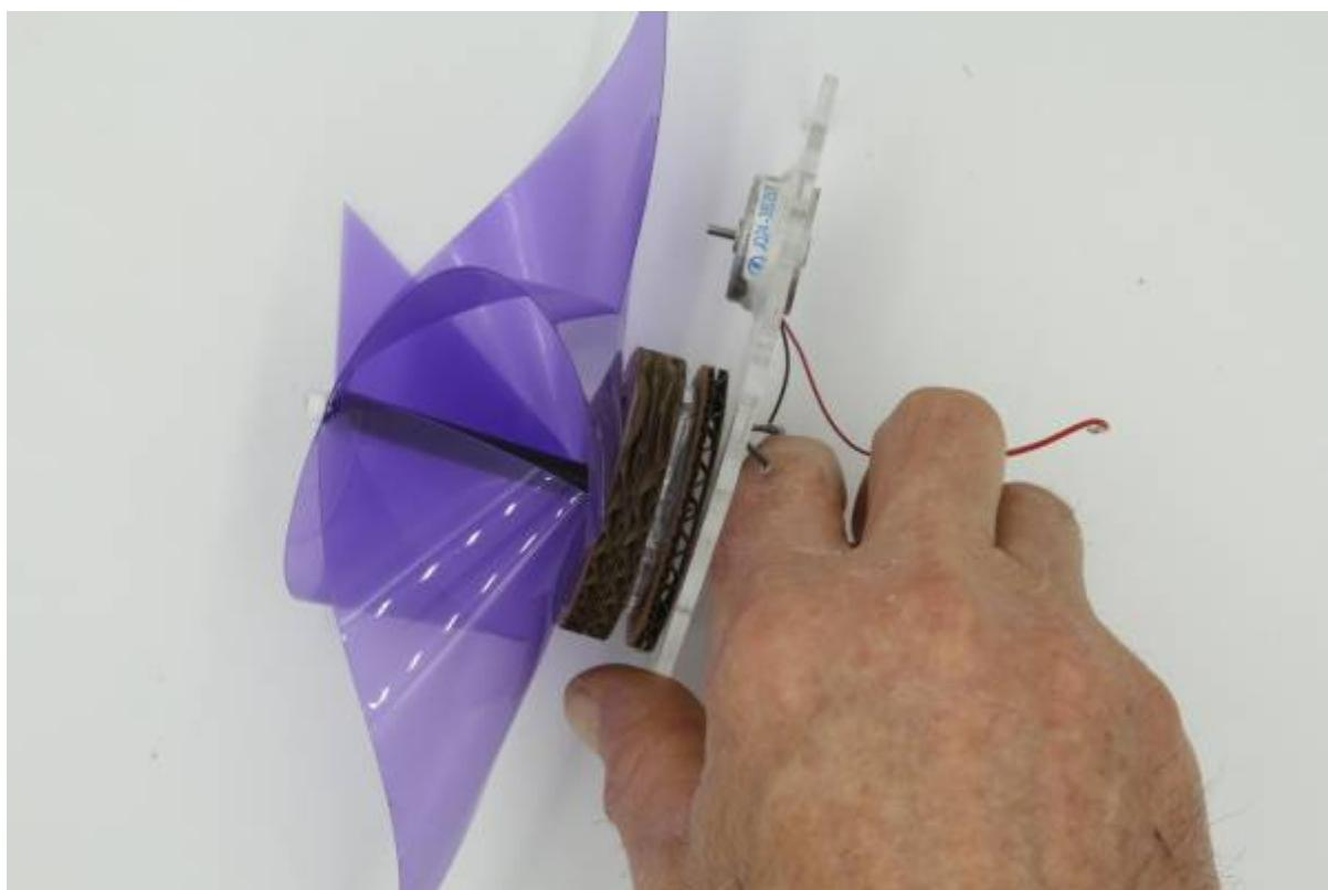
Slide the spinner onto the axle, and check that the acrylic spinner hub aligns with the motor. Trim the spacer if necessary.
