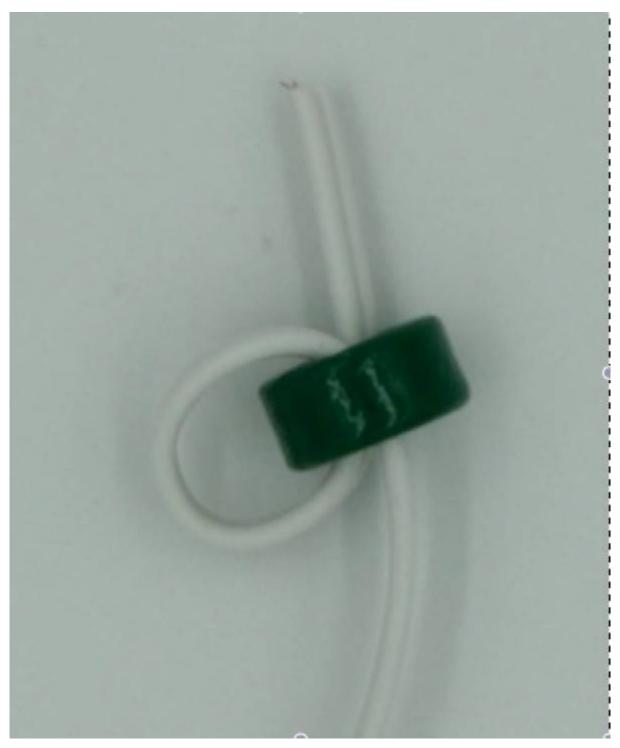
Using about 150mm of double wire (this depends on the size of your toroid), thread through the toroid taking care to avoid crossing over the strands. 5 or 6 loops are sufficient.
