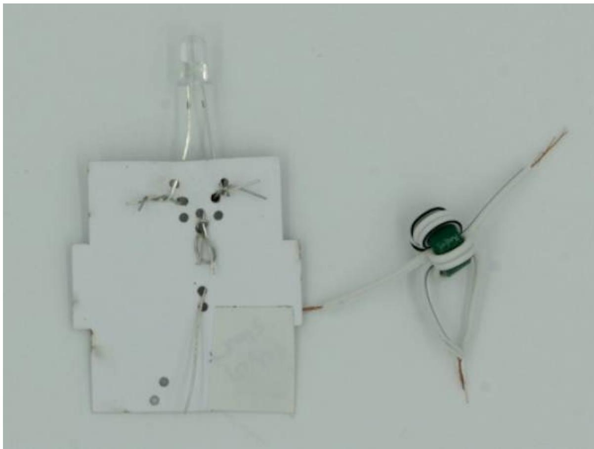
Attach the LED, taking care to put the longer leg on the right side. Twist together with the transistor on the back of the template.
