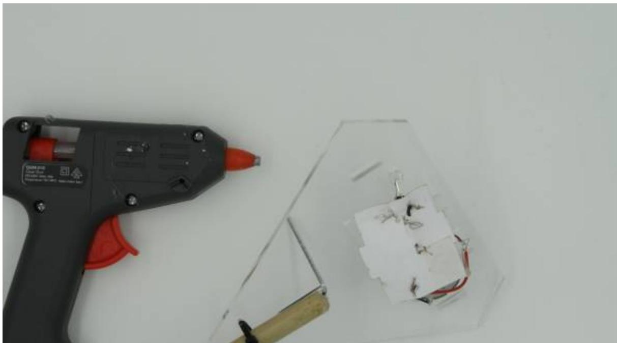
From the back of the chassis, insert the LED into the hole provided, and glue it in place.
