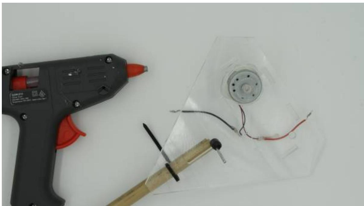
Glue the motor in the hole provided in the acrylic chassis with the shaft poking through (the motor should be on the left side, looking from the front).
