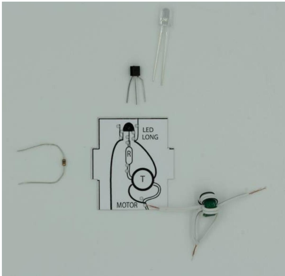
The circuit requires a NPN transistor, a 1K resistor, the wound toroid and an LED. Red LEDs work best, but yellow or green will also suffice.
