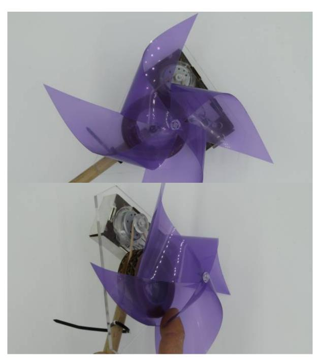
Take the rubber band, and loop it over the hubs so that it sits in the groove made by the acrylic hub. Now slide the 10mm spacer on to the axle, and then the spinner with the double hubs closest to the chassis.
