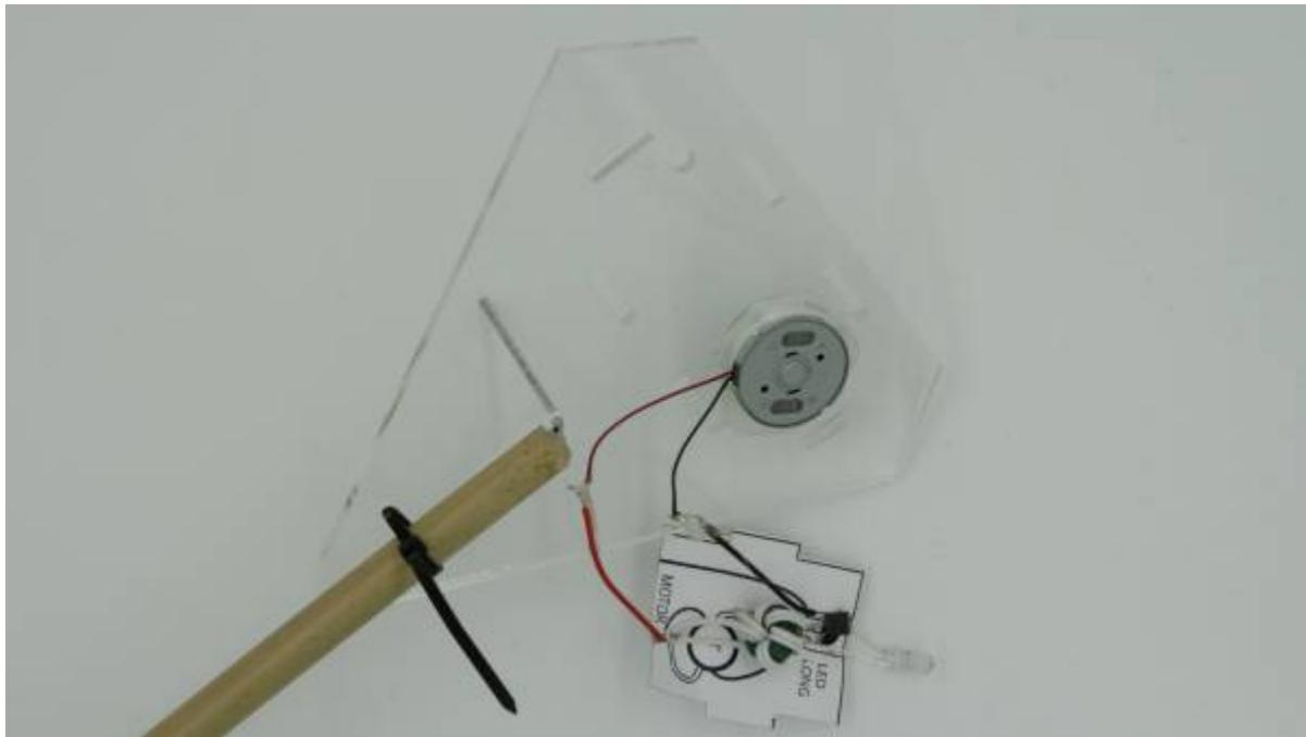
Now attach the motor wires as indicated: black wire to the transistor + LED, and red wire to the joined toroid wires.
