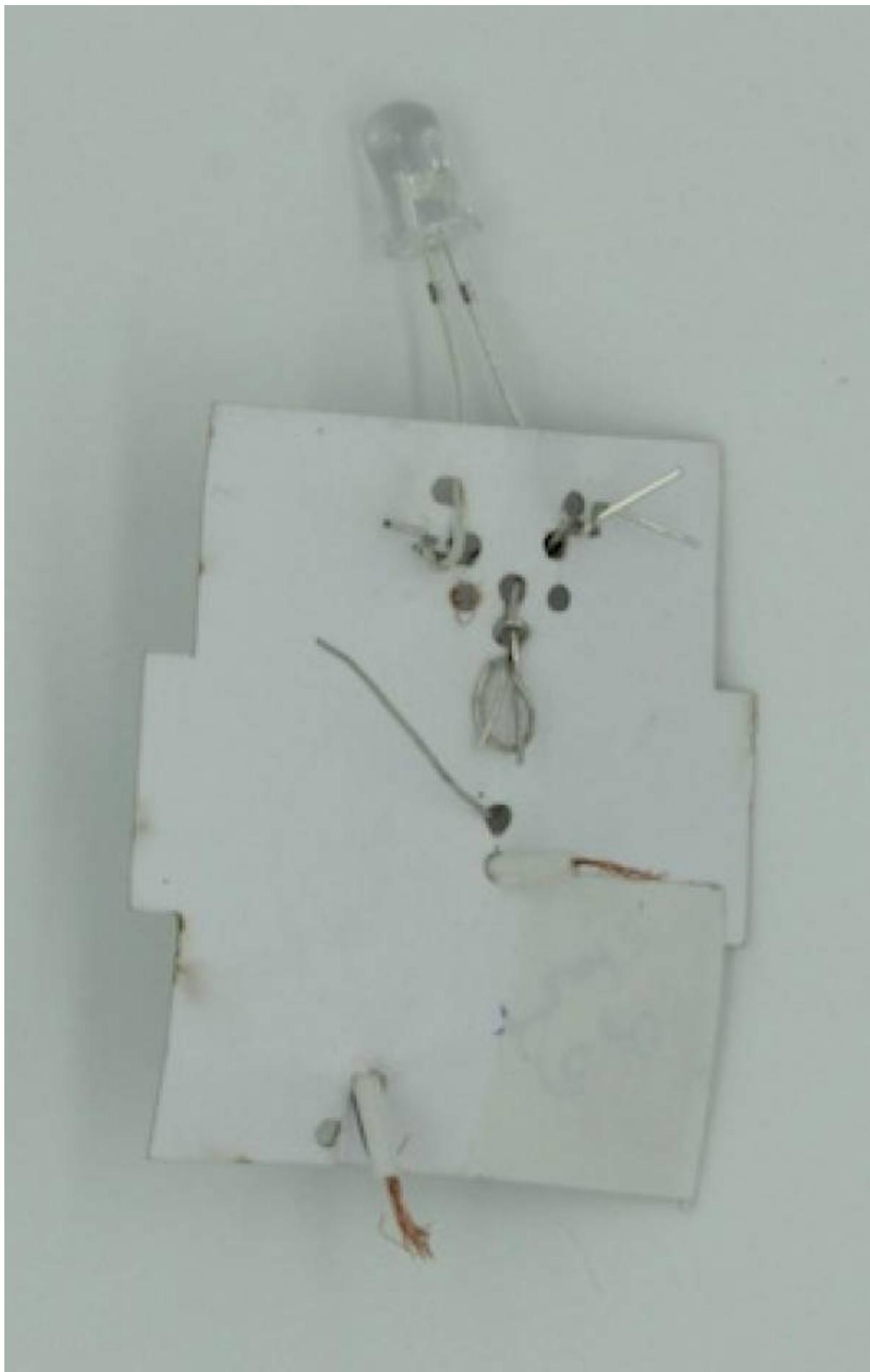
Finally , attach the toroid by pushing wires through the holes in the template and twisting together on the back.
