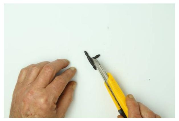
Use a craft knife to carefully cut the flanged end from the the centre of a T-shaped 4mm drip irrigation joiner.
