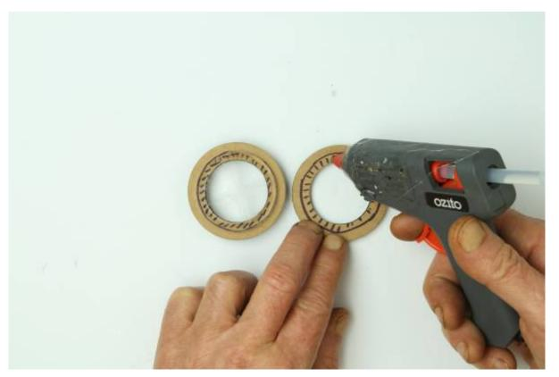
Now take the remaining cardboard hub, apply glue inside the etched area, and glue it to the acrylic hub.
