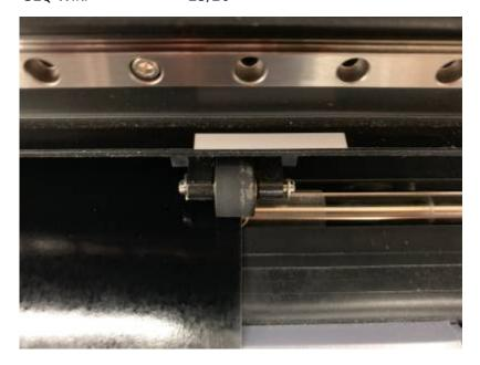
You also need to make sure the size of your print job will not exceed the size of the vinyl roll. When you feed the vinyl into the machine and hit enter, it should auto calculate the width and show on screen. Since we're just making small stickers, we should be fine but always good to check these settings.
